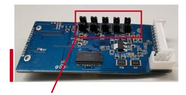
Five US imported sensors detect the output point position in real time during the handle working, effectively preventing multi-point overlay
